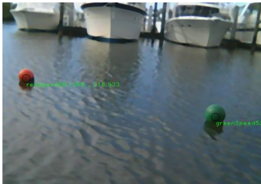
Figure 11 - Object detection (red thresholding also performed)
